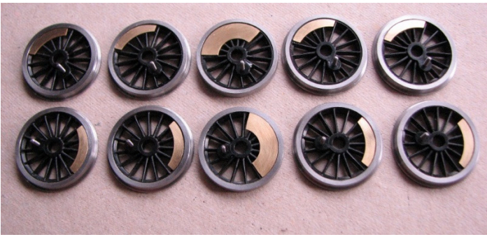
Wheels complete with weights and crankpins.
