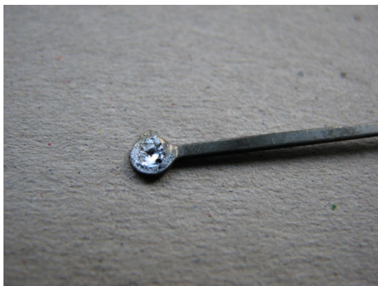
The resulting central dimple after over enthusiastic soldering.
